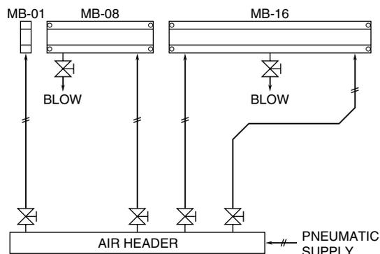
Select an appropriate pipe size for the required flow volume. Connect a stopping valve at the pipe connection to the air header for easy testing and maintenance.
