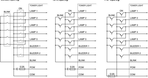
Note 1: Do not set lamp ON input to "On" and BLINK input to "Blink" at the same time watsoever, it might result in shortcircuit.
