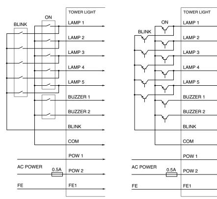
Note 1: Do not set lamp ON input to "On" and BLINK input to "Blink" at the same time watsoever, it might result in shortcircuit. Note 2: In order to improve EMC performance, bond the FE1 terminal to ground. Caution: FE1 terminal is NOT a protective conductor terminal.
