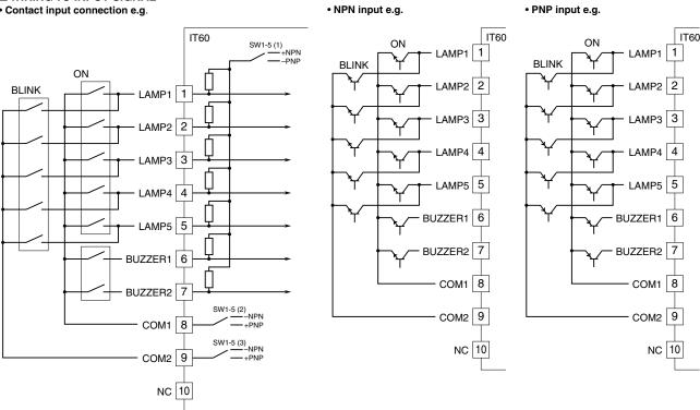
Note 1: SW1-5 turns on NPN input and contact input; PNP input tuns off SW1-5 input.
