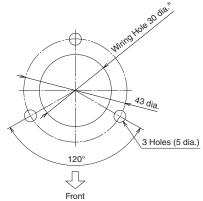
\* Protect wires to prevent scratching them at the edge of the compartment.
