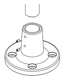
• Remove a rubber bush to insert a cable of large diameter, such as extended LAN cable (model: ITCA).
