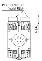
Input shunt resistor attached for current input.
