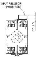
Input shunt resistor attached for current input.
