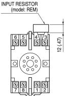
Input shunt resistor attached for current input.
