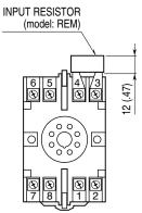
Input shunt resistor attached for current input.
