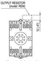
Use output shunt resistor for voltage output.
