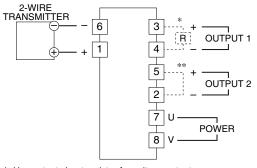
\* Use output shunt resistor for voltage output.
