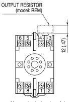
Use output shunt resistor for voltage output.
