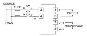
\* The transducer can be powered from the input voltage when the voltage is sufficiently stable and meets within the range of auxiliary power supply of the unit specified in the data sheet/instruction manual.
