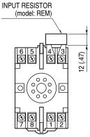
Input shunt resistor attached for current input.
