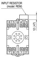
Input shunt resistor attached for current input.
