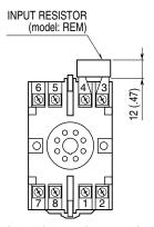
Input shunt resistor attached for current input.
