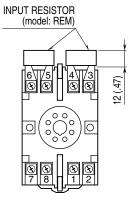
Input shunt resistor attached for current input.
