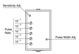
Positions for the rotary switches  $10^{-1}$  through  $10^{-n}$  apply respectively to each digit of the decimals and exponential as shown below.
