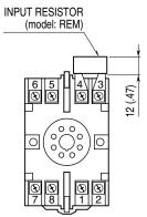
Input shunt resistor attached for current input.
