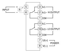
\*Input shunt resistor attached for current input.
