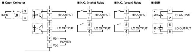
\*Input shunt resistor attached for current input.
