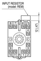
Input shunt resistor attached for current input.
