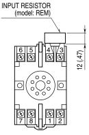
Input shunt resistor attached for current input.
