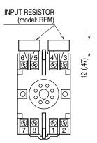
Input shunt resistor attached for current input.
