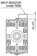
Input shunt resistor attached for current input.
