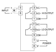
\*Input shunt resistor attached for current input.
