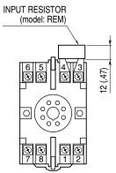
Input shunt resistor attached for current input.
