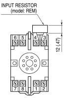
Input shunt resistor attached for current input.
