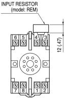
Input shunt resistor attached for current input.
