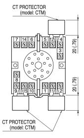
\*CT Protector (model: CTM) attached to these terminals. \*\*The transducer can be powered from the input voltage when the voltage is sufficiently stable and meets within the range of auxiliary power supply of the unit specified in the data sheet/instruction manual.
