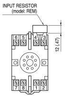
Input shunt resistor attached for current input.
