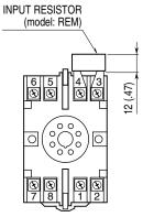
Input shunt resistor attached for current input.
