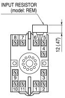
Input shunt resistor attached for current input.
