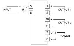
\*Input shunt resistor attached for current input.
