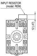
Input shunt resistor attached for current input.
