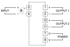
\* Input shunt resistor attached for current input.
