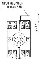
Input shunt resistor attached for current input.
