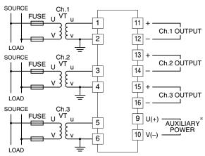
\* The transducer can be powered from the input voltage when the voltage is sufficiently stable and meets within the range of auxiliary power supply of the unit specified in the data sheet/instruction manual.
