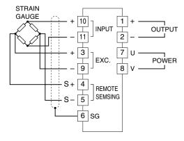
Close across the terminal 3-4 and 5-9 when the remote sensing is not used.
