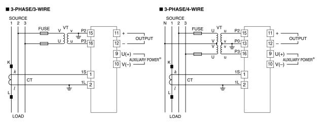
\*The transducer can be powered from the input voltage when the voltage is sufficiently stable and meets other supply voltage requirements.
