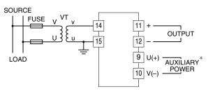
\*The transducer can be powered from the input voltage when the voltage is sufficiently stable and meets other supply voltage requirements.
