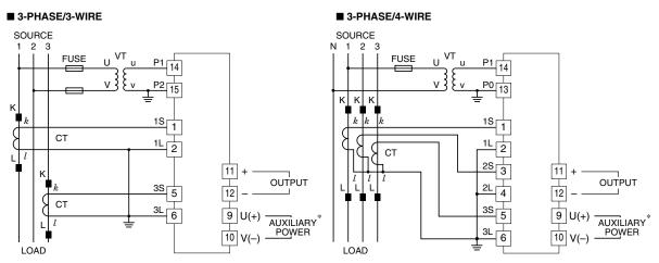
\*The transducer can be powered from the input voltage when the voltage is sufficiently stable and meets other supply voltage requirements.
