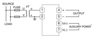
\*The transducer can be powered from the input voltage when the voltage is sufficiently stable and meets within the range of auxiliary power supply of the unit specified in the data sheet/instruction manual.
