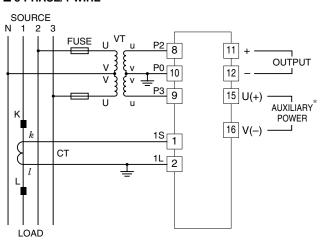
\*The transducer can be powered from the input voltage when the voltage is sufficiently stable and meets within the range of auxiliary power supply of the unit specified in the data sheet/instruction manual.
