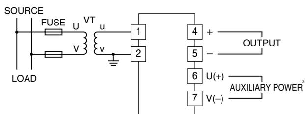
\*The transducer can be powered from the input voltage when the voltage is sufficiently stable and meets within the range of auxiliary power supply of the unit specified in the data sheet/instruction manual.
