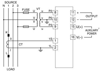
\*The transducer can be powered from the input voltage when the voltage is sufficiently stable and meets within the range of auxiliary power supply of the unit specified in the data sheet/instruction manual.
