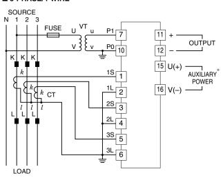
\*The transducer can be powered from the input voltage when the voltage is sufficiently stable and meets within the range of auxiliary power supply of the unit specified in the data sheet/instruction manual.
