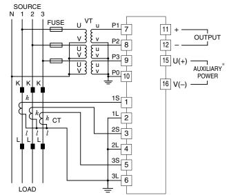
\*The transducer can be powered from the input voltage when the voltage is sufficiently stable and meets within the range of auxiliary power supply of the unit specified in the data sheet/instruction manual.
