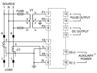
Pulse Output Connection Example Open Collector
