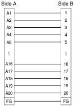
Pins No. B1 - B20 on Side A are not connected.
