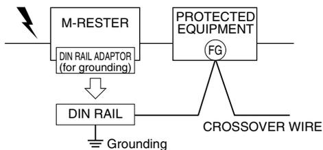
Cross-wire from the DIN rail to the metal housing of the protected device to equalize the ground potential.
