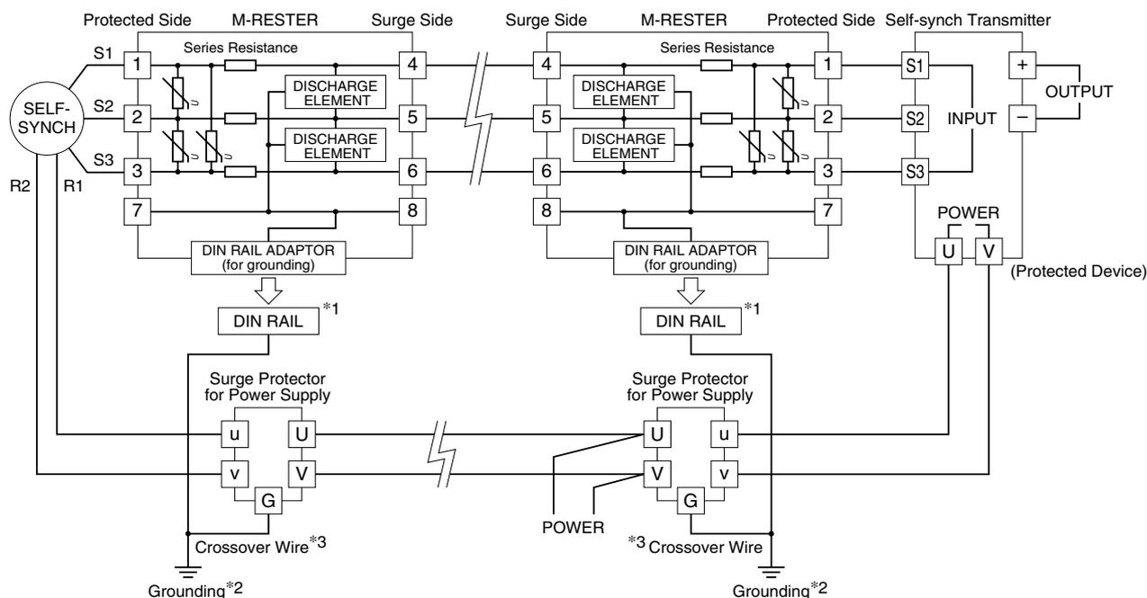
\*1. Oxide coating of an aluminium rail may lower the electric conductivity between this module and the ground. Use a steel or copper rail.
