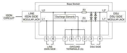
Be sure to cross-wire between the G terminal of telephone set and one of the terminals 7, 8, 1, or 2 of the MD-INS.
