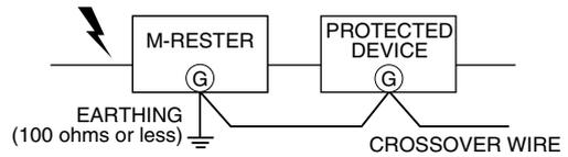
A crossover wire between M-RESTER earth and the earth or metallic housing of the equipment is required for protection. If the protected equipment has no earth terminal, earth the M-RESTER only.
