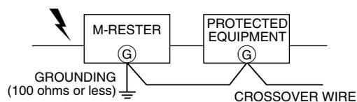
A crossover wire between M-RESTER ground and the ground or metallic housing of the equipment is required for protection. If the protected equipment has no ground terminal, ground the M-RESTER only.
