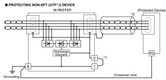
\*1. Maintain the shortcircuit bar. The protected device is 'grounded.'
