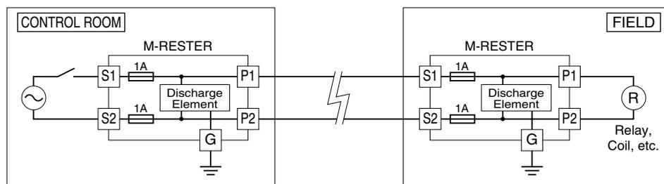
The M-RESTER must be connected with its terminals S1 and S2 faced on power source side in order that the fuses would be blown in case of shortcircuit of the discharge element.
